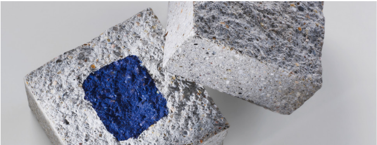
Protectosil® products offer deep penetration into the substrate resulting in a protective barrier that forms from within the structure
